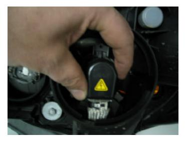
Figure 6a HID Socket (Locked)
