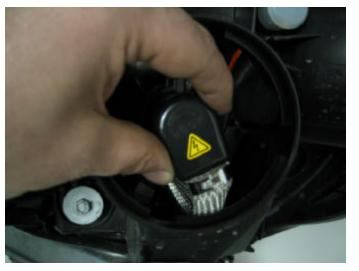
Figure 6b HID Socket (Unlocked)
