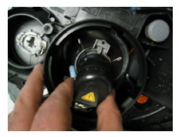
Figure 7 Pull to Remove
