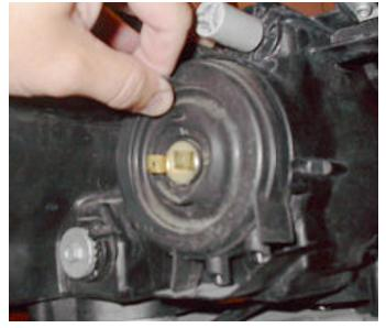
2. Remove the rubber cap over the High beam bulb (Part Number 10).
