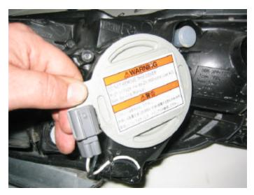
5. Remove the "Danger High voltage" cover. Each cover is marked with direction for Lock and Unlock.
