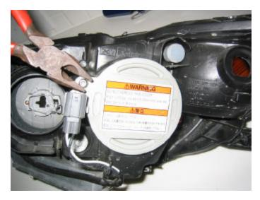
Figure 4 Security Screw Removal T25
